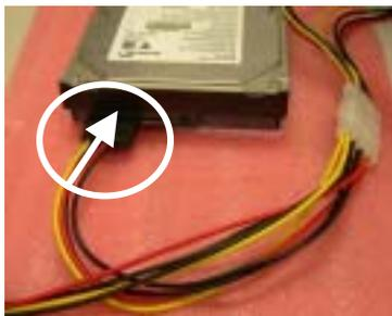
**Step 4.** Connect SATA data cable to the SATA HDD.
