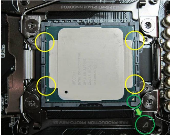
**Step 3. Close the socket:** Press down the levers on both sides, and secure them under the retention tab. The protection cover will automatically come off by itself.
