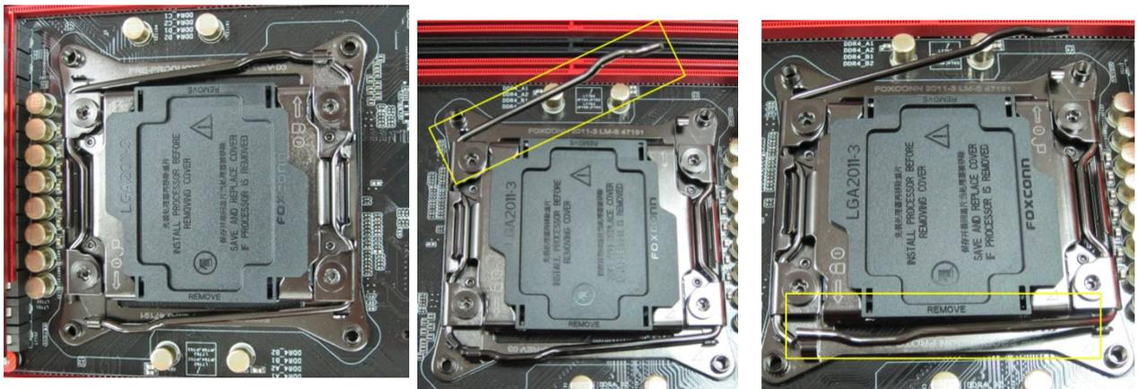
Step 2. **Insert the LGA 2011-3 CPU:** Make sure that you locate Pin1 and the two orientation key notches to where they belong, and then carefully place the CPU into the socket.
