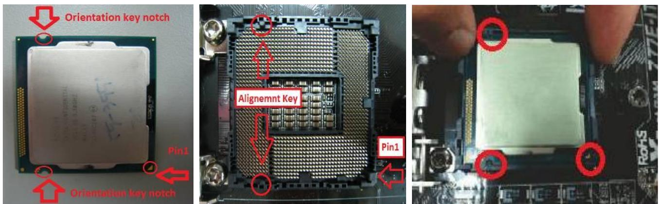
**Step 3. Close the socket:** Press down the load lever, and secure it with the load plate tab under the retention tab. The protection cover will automatically come off by itself.
