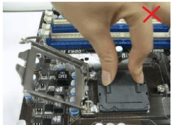
NEVER remove PnP Cap as pictured on the below. Incorrect removal of the PnP cap may cause damage to the CPU socket contacts.
