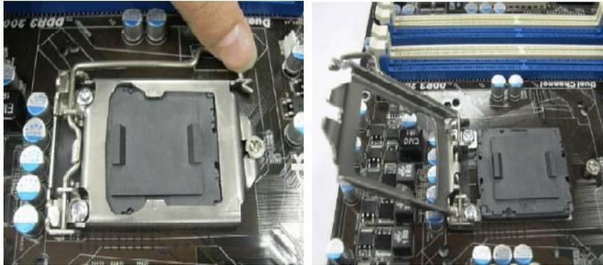
**Step 2. Remove CPU protection cover:** Attach your index finger to the upper edge of the PnP Cap. Use your thumb to remove PnP Cap (Pick and Place Cap) from the CPU socket by lifting the **cap tab**.
