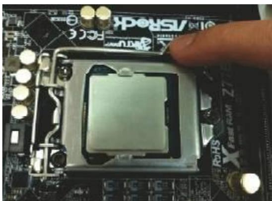
**Type B: CPU protection cover in CPU socket.**
