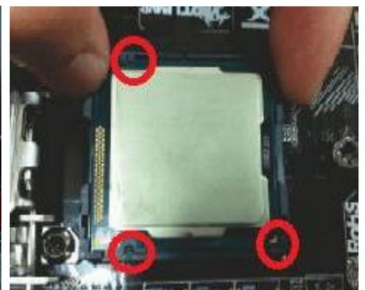
**Step 4. Close the socket:** Press down the load lever, and secure it with the load plate tab under the retention tab.
