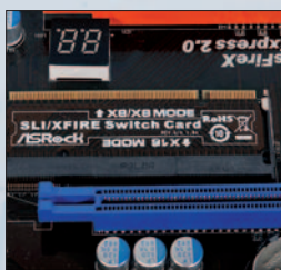
The sideport SLI/XFIRE switch card allows for manual switching of x16 and x8 modes for the PCI-e lanes
