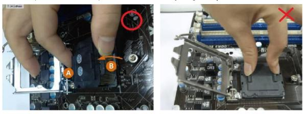
NEVER remove PnP Cap as pictured on the below. Incorrect removal of the PnP cap may cause damage to the CPU socket contacts.
