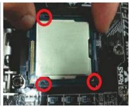
Step 3. Close the socket: Press down the load lever, and secure it with the load plate tab under the retention tab. The protection cover will automatically come off by itself.
