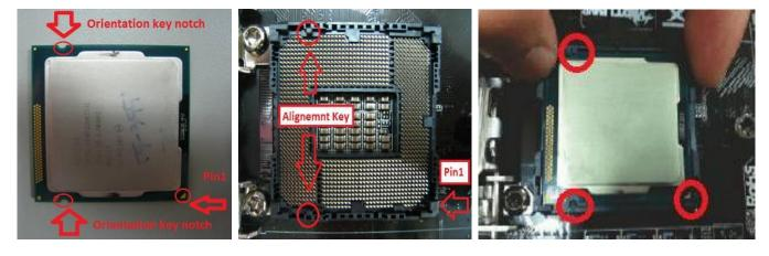
**Step 4. Close the socket:** Press down the load lever, and secure it with the load plate tab under the retention tab.
