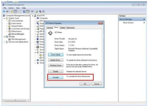
Step4. Enable "Delete the driver software for this device" option and then press "OK".
