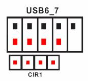
The properly connecting USB front panel cable with CIR header as below picture.
