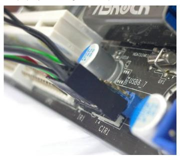
Step2: Please connect CIR receiver to USB front panel before booting up system.
