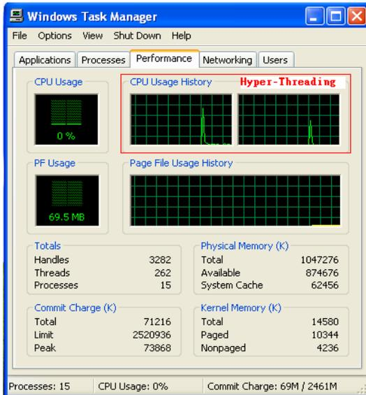
If you see only one figure of CPU Usage History, it means that the system is not working under Hyper-Threading. (Please refer to the following picture).
