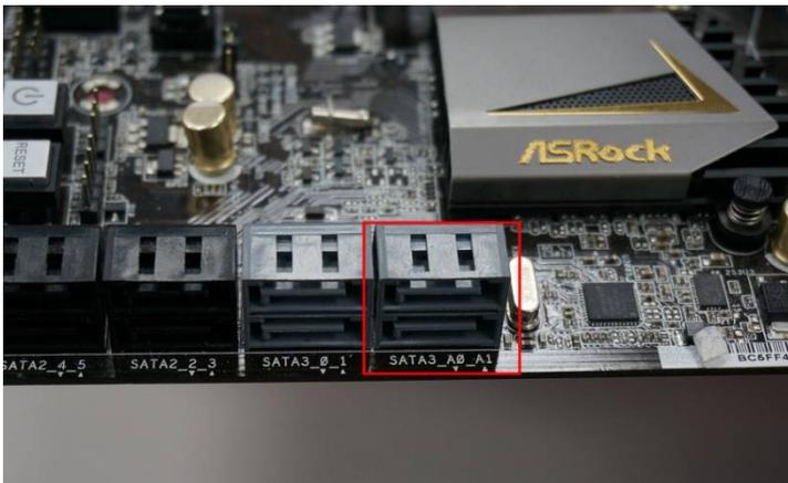
Or you could connect the HDD to SATA3\_0/ SATA3\_1 ports and install ASMedia SATA3 driver again.
