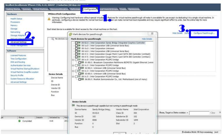
17. If VT-d feature is not able to use, the "Configure Passthrough Device" option will be gray, and showing the error message "Host does not support passthrough configuration" as below.
