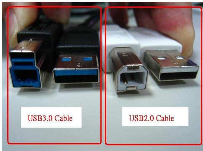
If you connect USB2.0 cable on USB3.0 external HDD device like below, it will not run at SuperSpeed mode.
