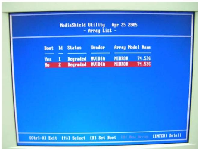
**Step 2:** Press “Enter” to get into the “Array Detail”
