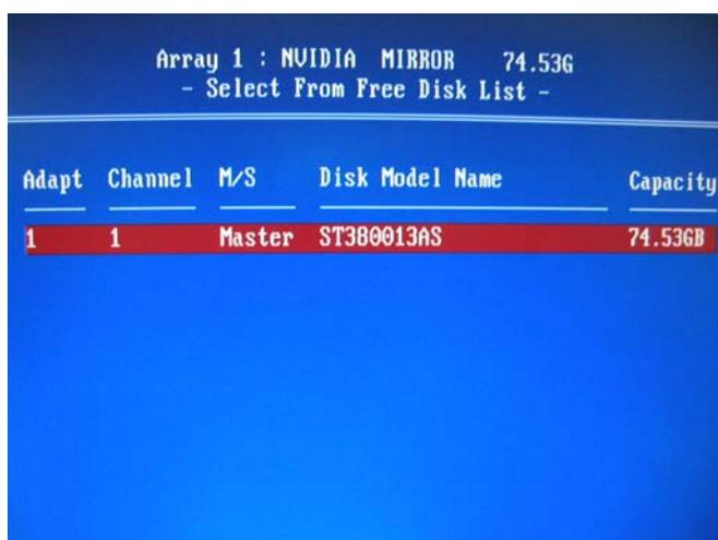
**Step 6:** Press “A” then “Enter” to rebuild array.
