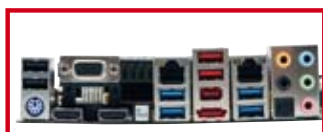
The Clear CMOS button sits between the Multi-VGA output ports and PCIE GLAN ports
