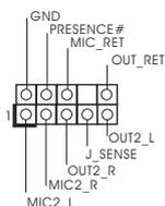
This header is for connecting audio devices to the front audio panel.
