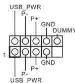
There are two headers on this motherboard. Each USB 2.0 header can support two ports.
