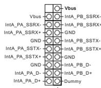
There is one header on this motherboard. Each USB 3.0 header can support two ports.
