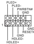
Connect the power switch, reset switch and system status indicator on the chassis to this header according to the pin assignments below. Note the positive and negative pin before connecting the cables.
