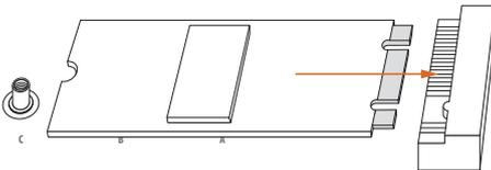
Align and gently insert the M.2 (NGFF) SSD module into the M.2 slot. Please be aware that the M.2 (NGFF) SSD module only fits in one orientation.
